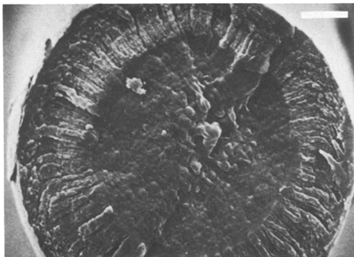
Figure 13 SEM of tensile fracture of 10 Mrad gamma-irradiated nylon 6 fibre, fractured in air (5 \mu\text{m} bar).
